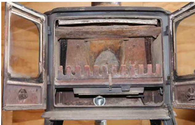
Fig 1. Cold air intake at the back of the ash compartment underneath the firebox (ash tray removed) after a few months of use. Note a shiny appearance of the duct with no trace of smoke presence. The stove is 10 years old.
