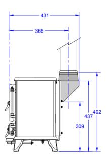
Please note that the Rear Flue Wedge is to be classed as single wall flue pipe so in this case requires the following clearances:
