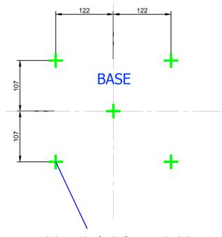
Mark the position for the four mounting bolts on the hearth.
